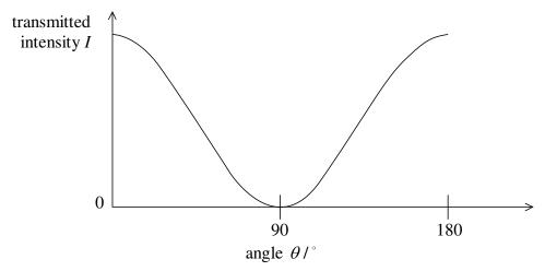
solution placed between two crossed polarizer; plane of polarization rotated by an amount that depends on concentration; rotation of second polarizer/intensity of transmitted light is a measure of
